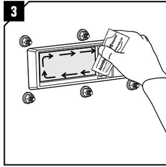
Lubricate the inside surfaces of the frame with Roxtec Assembly Gel, especially in the corners.
