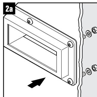
Attach the frame firmly, using the enclosed screws, washers and nuts.
