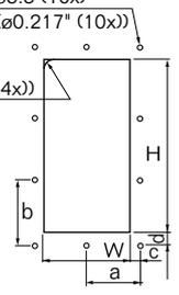
Cut a rectangular opening for the frame, according to the tables above. For Roxtec ComSeal™ 12 cut a rectangular opening according to FL 21 or the table above.
