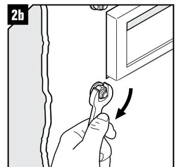
Tighten the nuts firmly, crosswise and in small steps.
