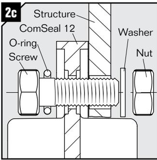
For ComSeal 12, attach the frame firmly, using the enclosed screws, nuts, o-rings and washers. Make sure that the o-ring is mounted under the bolt head.
