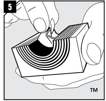
Adapt the modules, which are to hold cables or pipes. Peel off layers until you achieve the gap seen in step 6. The halves may not differ by more than one layer.
