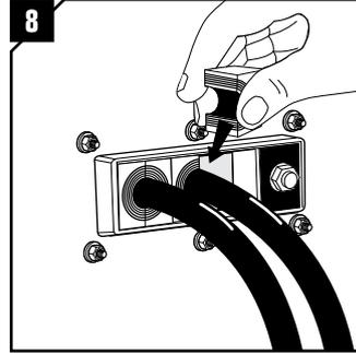
Insert the modules from the back of the frame opening and according to the installation plan (Packing plan). If possible, start with the largest modules.
