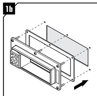
Alternatively, insert it with the other side of the flange and gasket facing the wall/structure.
