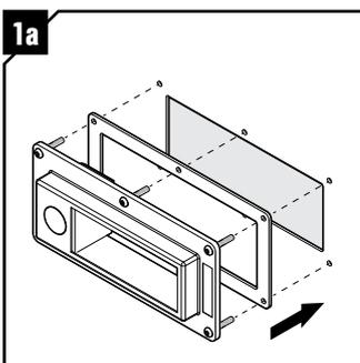
Insert the frame in the opening with gasket side towards the wall/structure. Use the screws for keeping the gasket in place.
