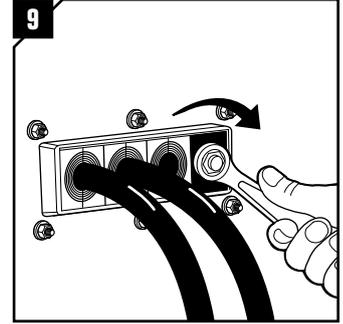
Tighten the compression unit firmly to seal the frame. Maximum 10 Nm (7.38 ft. lb). A good indication is when the assembly gel is squeezed out between the modules.
