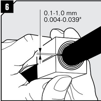
Achieve a 0.1-1.0 mm gap between the two module halves when held against the cable/pipe.
