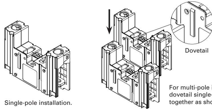
**NOTE:** Installation requires two (2) #6-32 x 1-3/4" customer supplied mounting screws per pole and desired lug kit (see table on next page).
