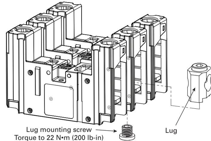
Installing lug kit catalog numbers CCP2-L4-1 and CCP2-L4-1A for use on 400 amp holders
