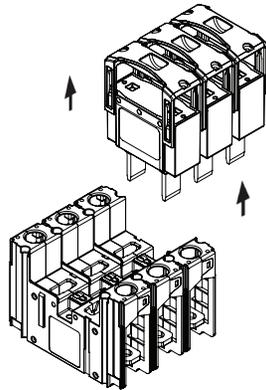
Extract fuses by extending built-in handles and pulling straight out.
