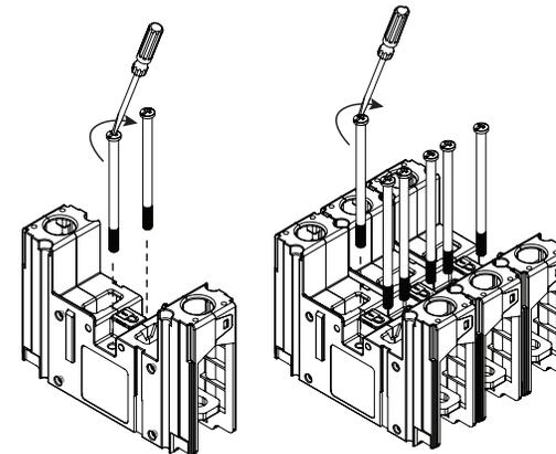
Locate and mark holes for customer supplied mounting screws as shown. Drill and tap mounting holes in the back plate, insert mounting screws and torque to 2.3 N•m (20 lb-in).
