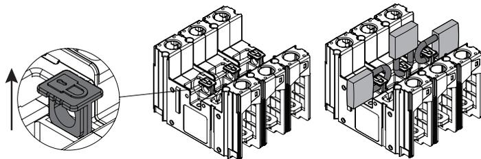
Lockout/tagout feature: pull tab out from base and insert one 1/4" lock per pole.
