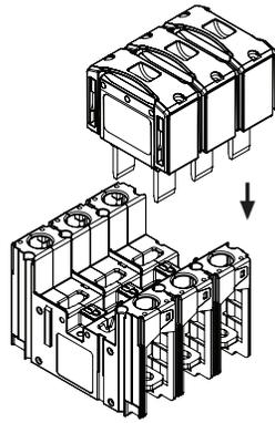
Insert fuses by aligning blades with holder slots and pushing in until fully seated.
