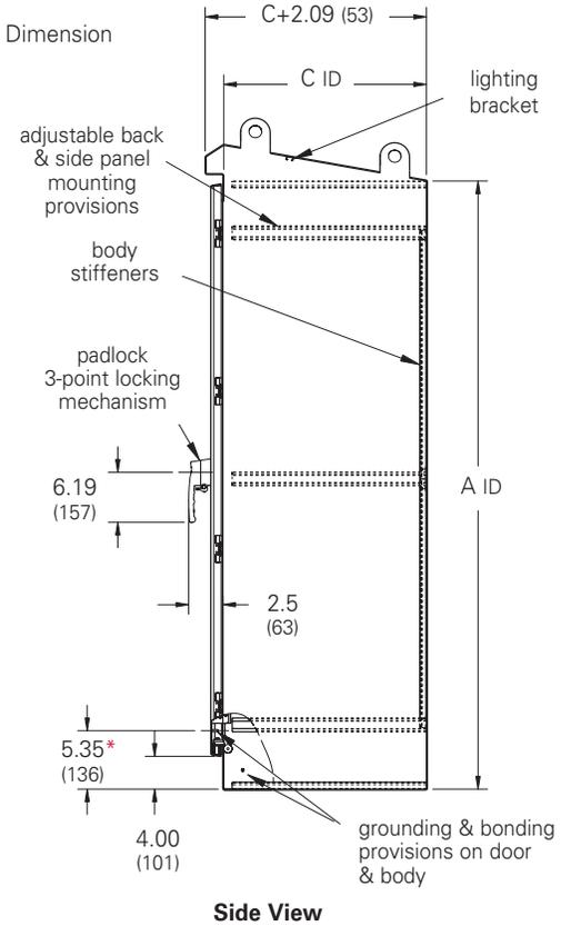
\* From flange opening to bottom of enclosure
