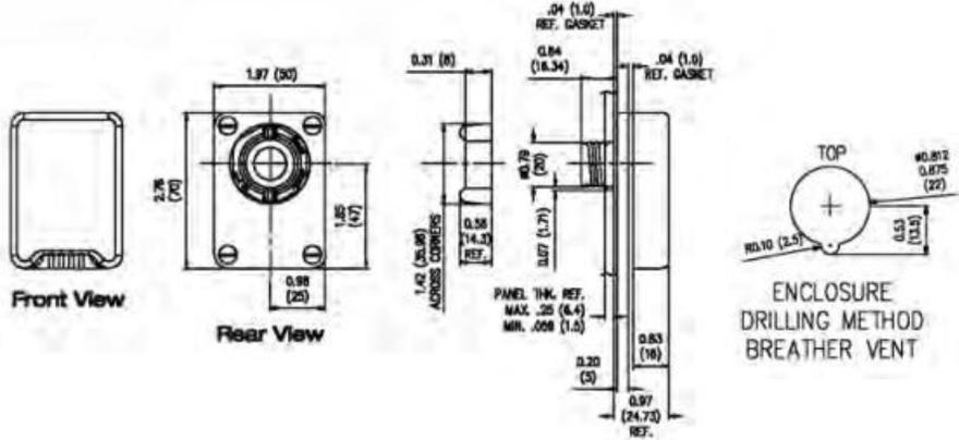
Non-metallic breather vent allows an enclosure to breathe, allowing the free passage of air while maintaining UL Type 4X enclosure integrity as a recognized component.
