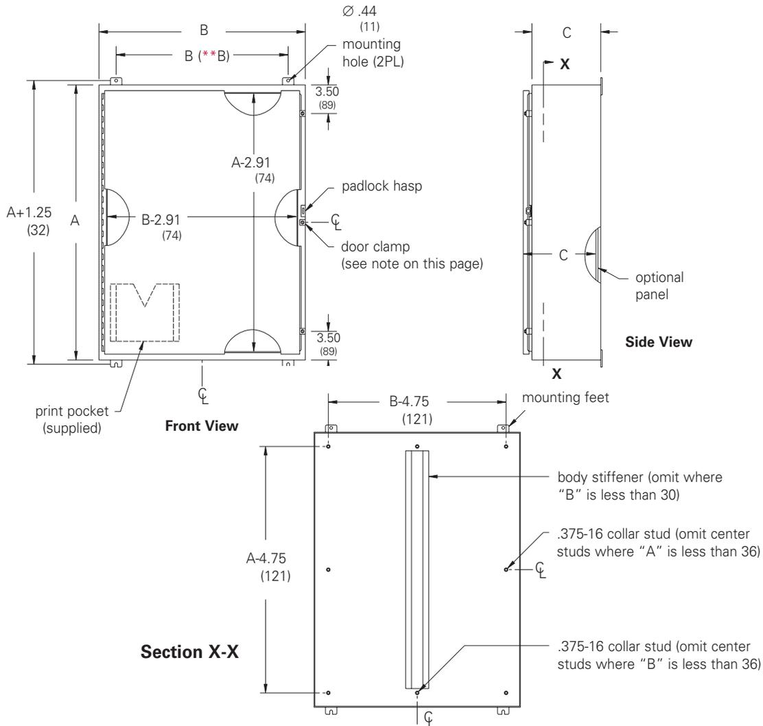
**Notes:** Dimensions: \*\*B = (-2.50) if 12 inches wide; (-6.00) if wider than 12 inches. Clamps are mounted along three sides of the enclosure door. Spacing between clamps along side opposite the hinge does not exceed 15 inches. Dimensions are in inches. Millimeters shown are for reference only. Data subject to change without notice.
