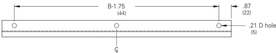
(omit center hole where "B" is less than 23.75)
