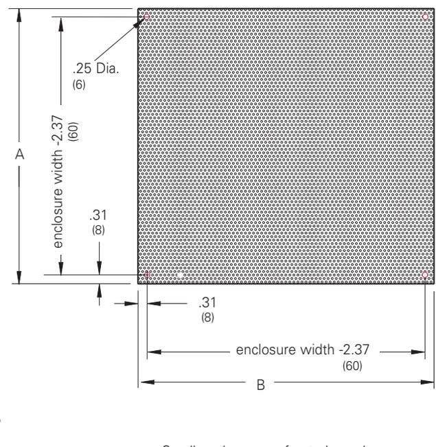
Small enclosure perforated panels can be installed in small Type 3R RHC, and small Type 1 Enclosures, and are intended for mounting lightweight components without drilling and tapping.
