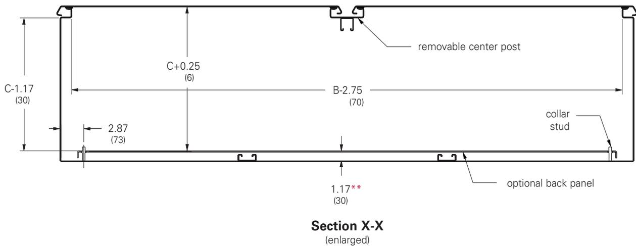
\*\* From top of panel stud flange to inside of enclosure
