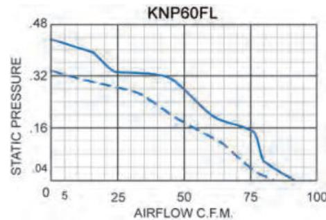
Airflow vs. static pressure curves are shown for 60 HZ and 50 HZ (broken line) inputs.
