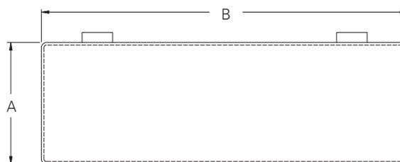
Intended for use with Type 12 Enclosures and is an excellent means of providing a removable access plate to an enclosure and still maintain its listing. The Gland Plate is constructed from (16) gauge steel and has ANSI 61 gray polyester powder finish. Fastening is done from the inside of the enclosure to prevent tampering. Hardware and instructions are included with the kit. UL Listed.
