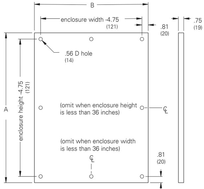
RHC Flat Panels can be installed in Large Type 3R RHC Enclosures. Panels are only available in steel and have a white powder paint finish.
