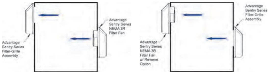
(Left) Filter Fan pressurizes cabinet. Filter-Grille Assembly exhausts cabinet.
