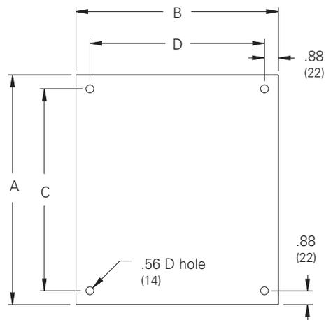
NEMA flat panels can be installed in Type 4X, Type 4 and Type 12 NEMA Enclosures. Panels are available in steel, galvanized steel, stainless steel, and aluminum. Painted steel panels have a white powder paint finish. Stainless steel and aluminum panels have a smooth brushed finish on one side and protected with PVC film.
