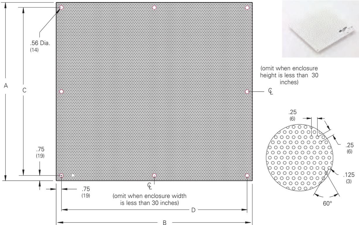
Type 1 medium enclosure perforated panels can be installed in Type 1 Medium Panel Enclosures. Panels are available in steel and have a white powder paint finish.
