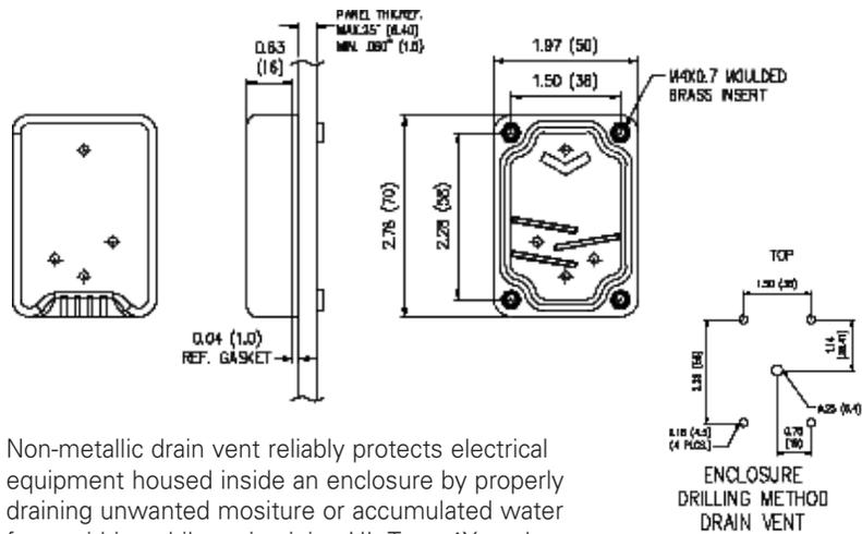
Non-metallic drain vent reliably protects electrical equipment housed inside an enclosure by properly draining unwanted moisture or accumulated water from within, while maintaining UL Type 4X enclosure integrity as a recognized component.
