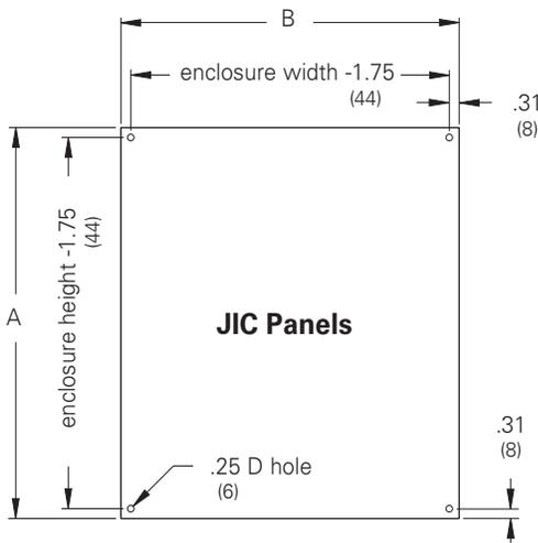
JIC panels can be installed in all types of JIC Enclosures. Some sizes will fit the NEMA 12 Lay-In Wireway Junction Box. Panels are available in steel, galvanized steel, stainless and aluminum. Painted steel panels have a white powder finish. Stainless steel and aluminum panels have a smooth brushed finish on one side and protected with PVC film.
