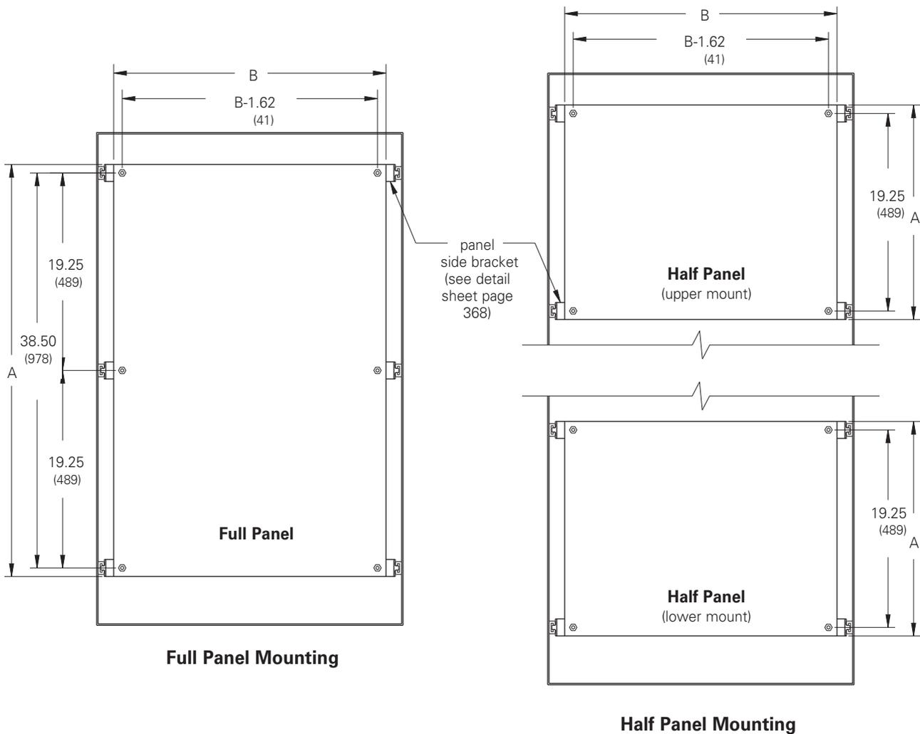
Full panel and half panel for consoles are (12) gauge steel and furnished with panel brackets and all hardware necessary for channel and panel mounting. Half panels can be mounted in either the upper or lower portion of the console. Console body design permits the panel to adjust along the depth of the enclosure. Full panel and half panel can be mounted back-to-back.
