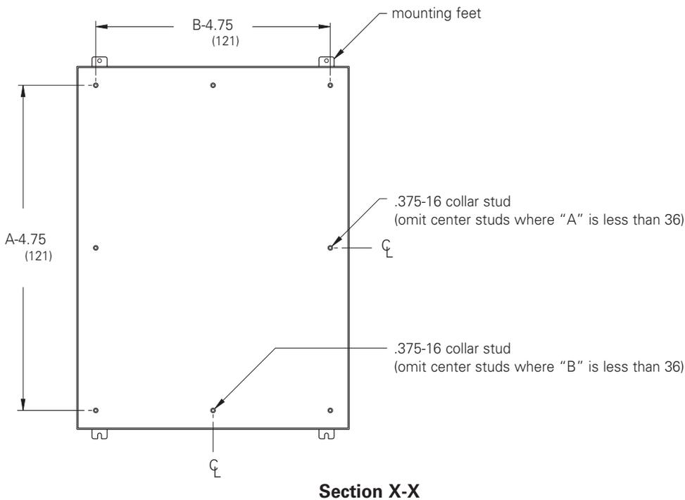
**Notes:** Dimensions: \*\*B = (-2.50) if 12 inches wide; (-6.00) if wider than 12 inches. Clamps are mounted along three sides of the enclosure door. Spacing between clamps along side opposite the hinge does not exceed 15 inches. Dimensions are in inches. Millimeters shown are for reference only. Data subject to change without notice.
