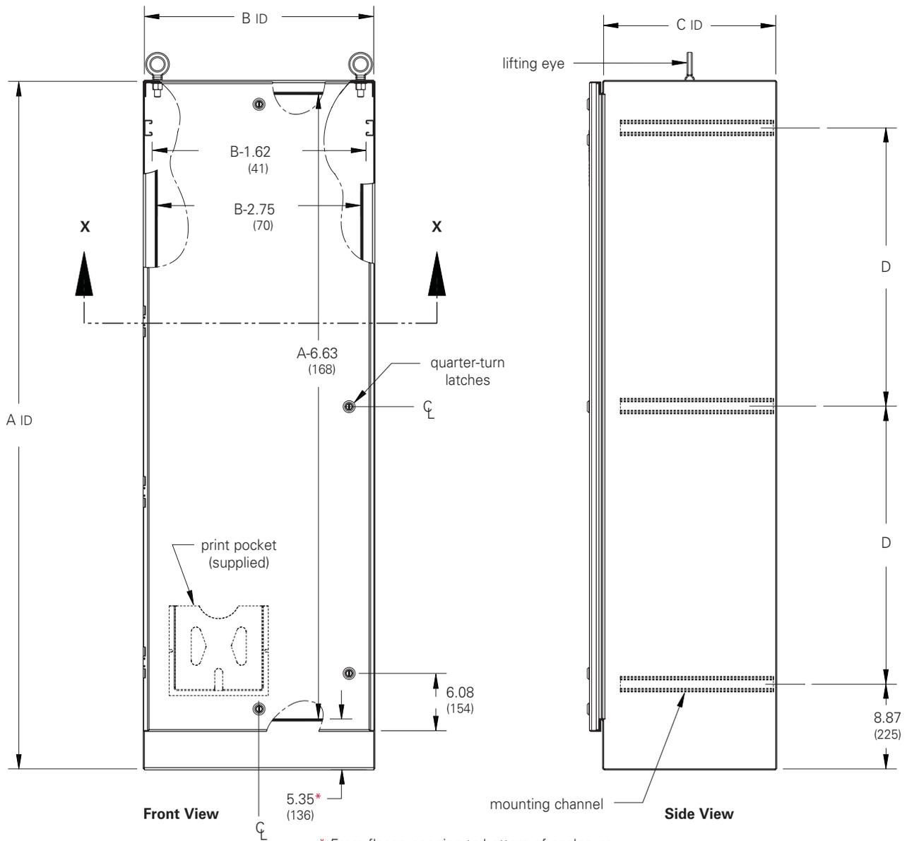
\* From flange opening to bottom of enclosure
