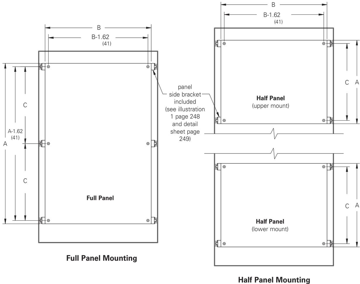
**Note:** Full and Half panel for single-door, single and dual-access enclosures are (12) gauge steel and furnished with panel side brackets and all hardware necessary for channel and panel mounting. Half Panels can be mounted in either the upper or lower portion of the enclosure. Free standing design permits the panel to adjust along the depth of the enclosure. With dual-access enclosures, Full and Half panels can be mounted back-to-back.
