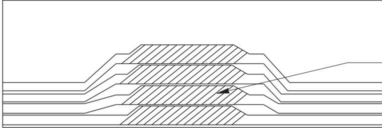
Cross sectional area of splices and taps is less than 75% of wireway's cross sectional area
