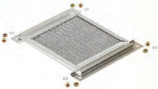
Designed for use with Louver Plate Kits. The Filter mounts securely inside of the enclosure using the brackets and hardware furnished with the kit. The Filter is comprised of finely woven aluminum strips which offers protection against airborne dust and dirt. Periodic washing with warm water is needed to keep the Filter clean.
