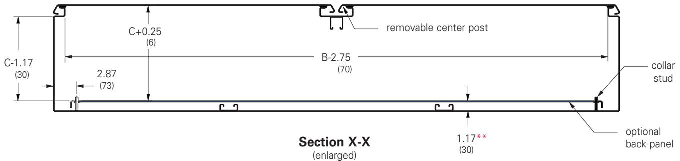
\*\* From top of panel stud flange to inside of enclosure
