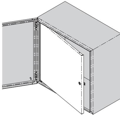
Note: Swing-out panel distance from panel face to inside of enclosure cover equals 1 1/4".
