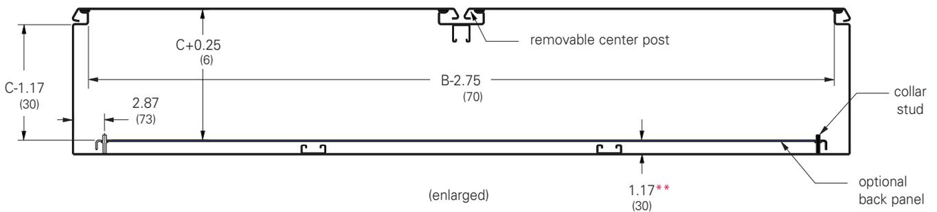
\*\* From top of panel stud flange to inside of enclosure
