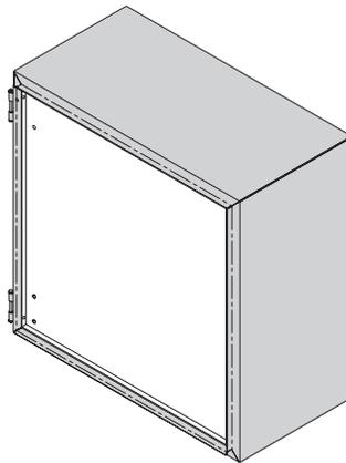
Note: Dead front panel distance from panel face to inside of enclosure cover equals 1 1/4".
